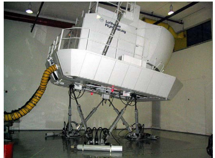
A Stewart Platform in use by Lufthansa
