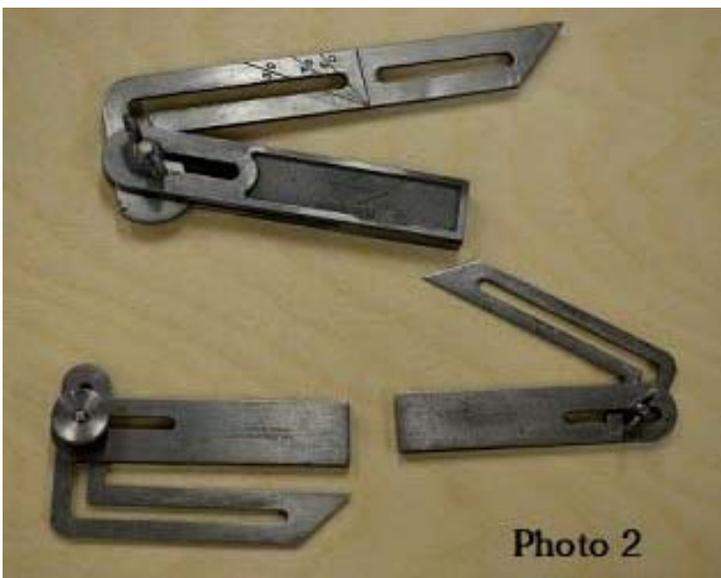
Photo 2 shows an assortment of three universal bevels I have in my tool chest. The smallest one and the middle size were made by Starrett. Brown & Sharpe made similar bevels. The largest bevel in Photo 2 is a cheap tool with a pot metal beam and a stamped steel blade made in the USA by TWIX a few decades ago.
