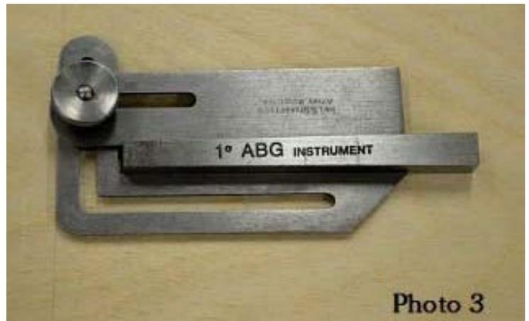
In Photo 3, you can see one of these bevels being used to measure a 1 degree angle, something that's not possible to do with a simple bevel. Another nice feature of universal bevels is that they will also measure any angle that can be measured with a simple adjustable bevel.
