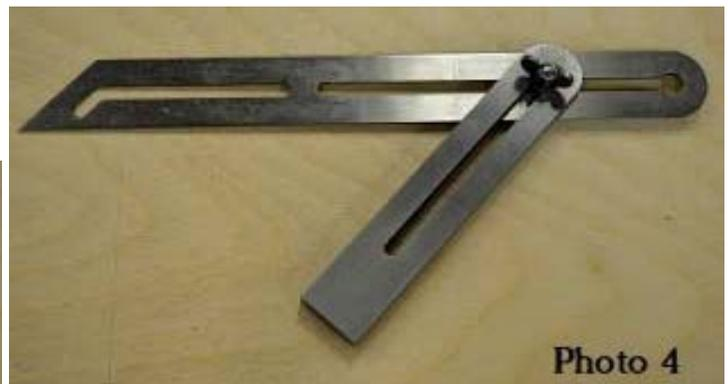
Photo 4 shows a "Universal Bevel" that is still in Starrett's catalog, but I don't think it's nearly as versatile as others. The "dog leg" section has been shrunken down to just a little jog in the blade slot, limiting its usefulness in measuring acute angles. Plus, it's a pain to move the beam from one slot to the other. And, trust me, the beam will always be in the wrong slot when you pick it up to use it.
