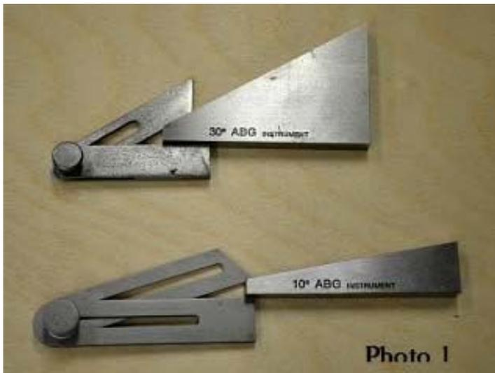
The simple bevel works fine at 45 degrees, but when you get down to 30 degrees, there's not enough contact area on the bevel's gauging surfaces to assure an accurate measurement. An acute angle of 10 degrees can't be measured at all. There were a few solutions developed to address this problem, but we are going to limit this discussion to the simplest one, the universal bevel.
