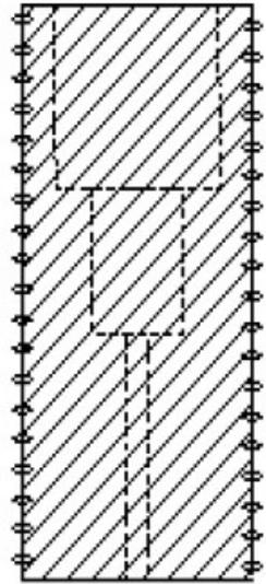
**Step 3 – thread in the slugs.** If you intend to leave it this way, use a bit of Loctite® on the threads before assembling. For better alignment, feed a close fitting rod through both slugs while the Loctite sets.
