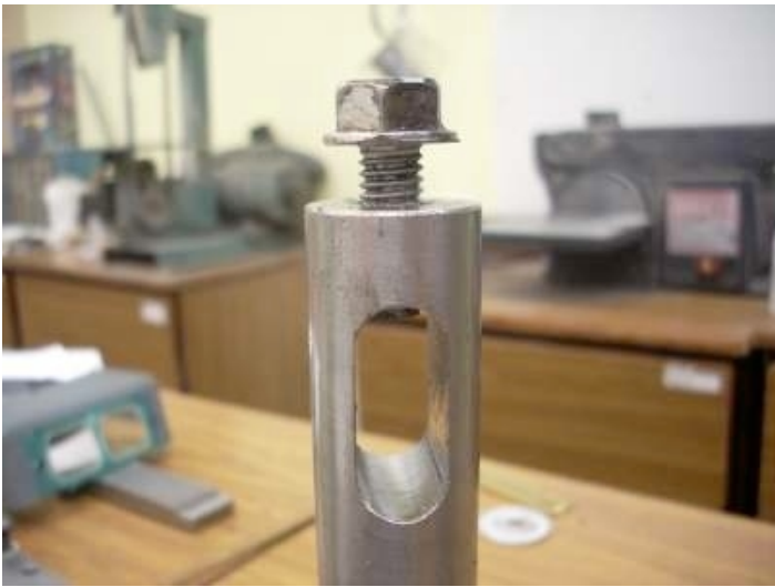
Slot Cut in Pivot Pin Photo by R. G. Sparber
