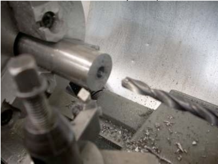
Drilling Pivot Pin Photo by R. G. Sparber
