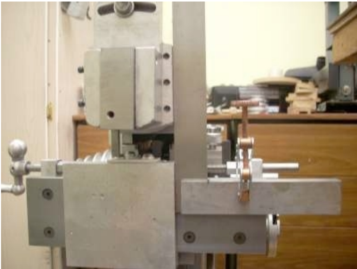
Aligning Head Photo by R. G. Sparber
