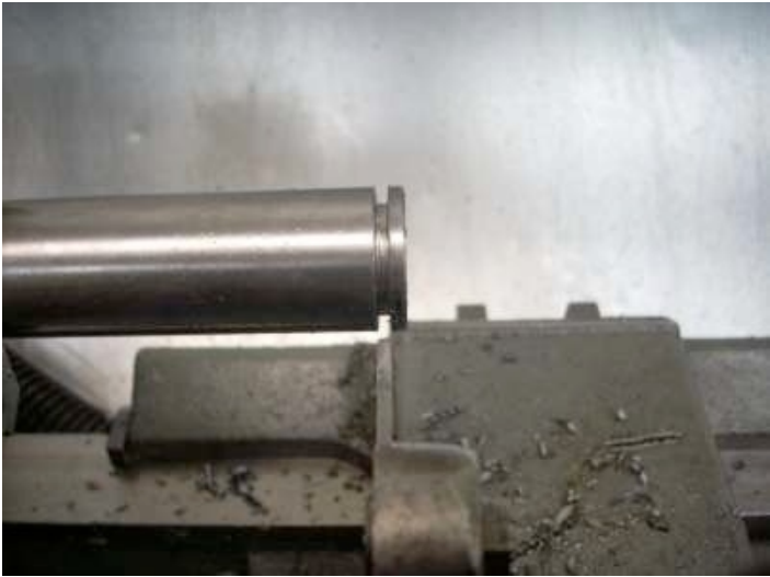
Groove Cut Photo by R. G. Sparber
