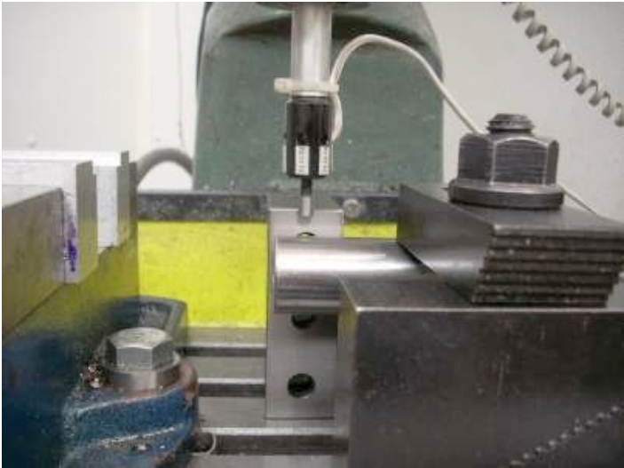
Locating Pivot Pin Center Photo by R. G. Sparber
