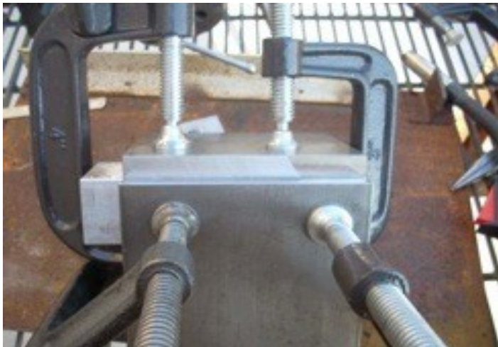
Clamped for Welding Photo by R. G. Sparber
