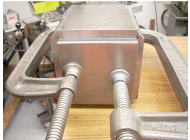
Backplate Clamped Photo by R. G. Sparber
