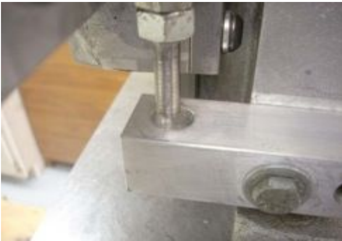
Fitting Lower Support Photo by R. G. Sparber
