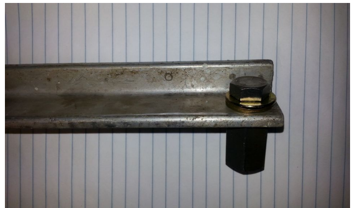
Figure 3 – Beam with 3/8" square drive on one end
