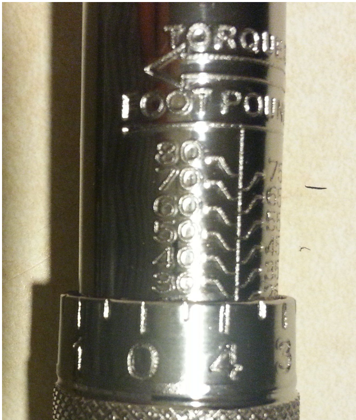
Figure 6 –Graduations On My 3/8" Torque Wrench Showing 29 Foot Pounds
