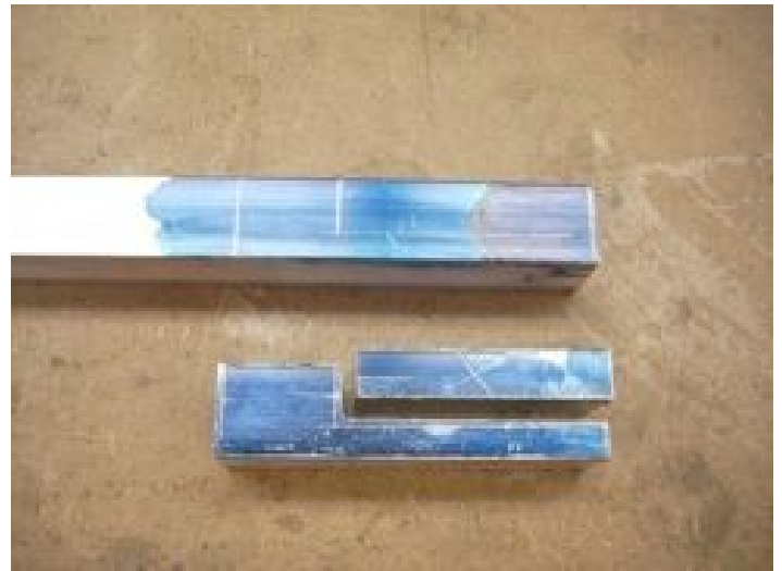
Bearing Supports Photo by R. G. Sparber
