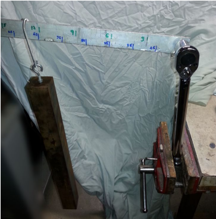
Figure 5 – Torque wrench being checked
