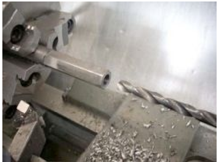
Drilling Nuts Photo by R. G. Sparber
