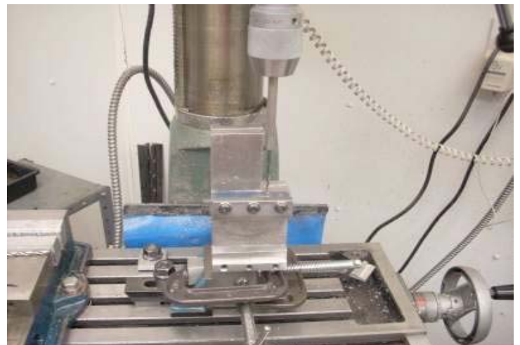
Drilling for Gib Screw Photo by R. G. Sparber
