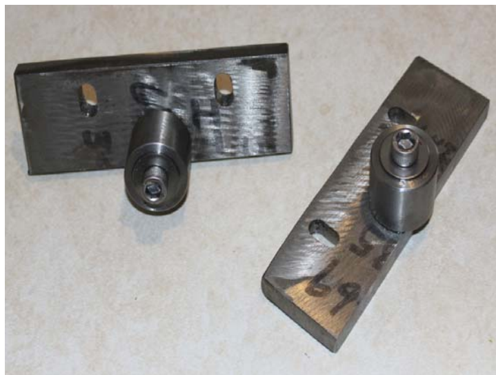
Figure 1 – Completed Stainless Rollers, Ready For Installation
