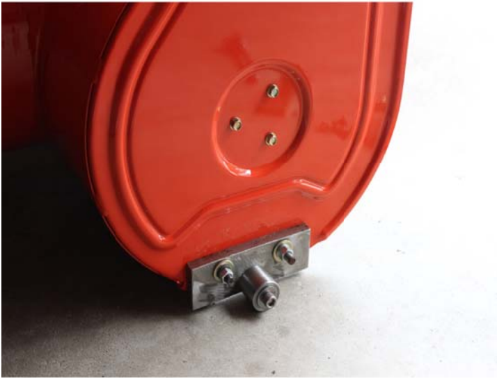
Figure 3 – Ariens Snowblower with Custom Stainless Rollers
