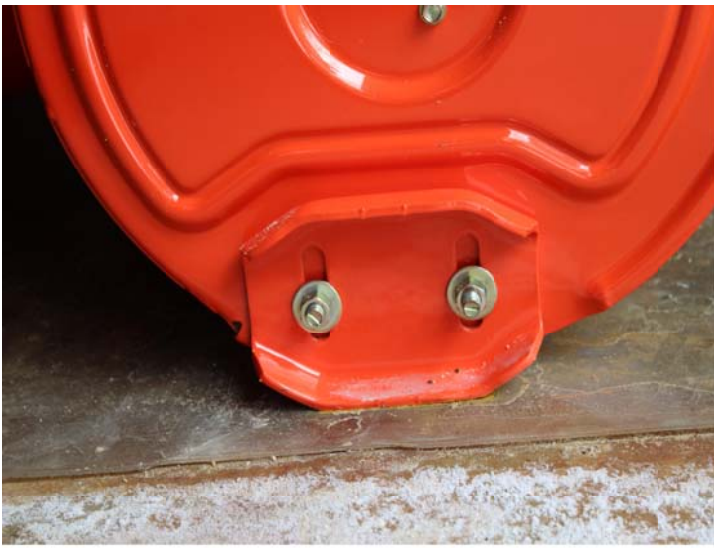
Figure 2 – Ariens Snowblower with Factory Skid Plates
