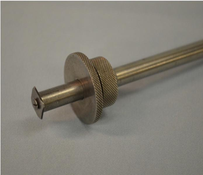
Note the different types of scribing points on these two gages. The classic gage has a round pin riveted in place with its hardened end sharpened to a conical point. Our example is typical of many of these older gages in that the pin has been sharpened nearly away over years of use to
