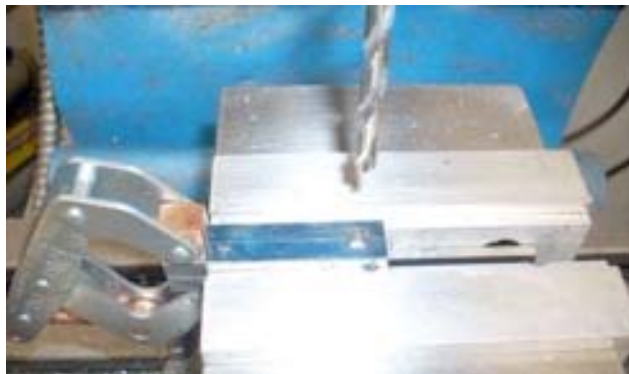
Drilling Links Photo by R. G. Sparber
