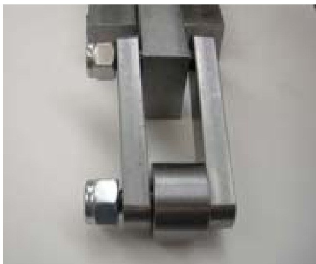
Link Assembly Photo by R. G. Sparber
