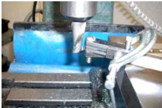
Rounding Link Ends Photo by R. G. Sparber
