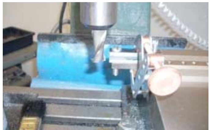
Milling Link Ends Photo by R. G. Sparber
