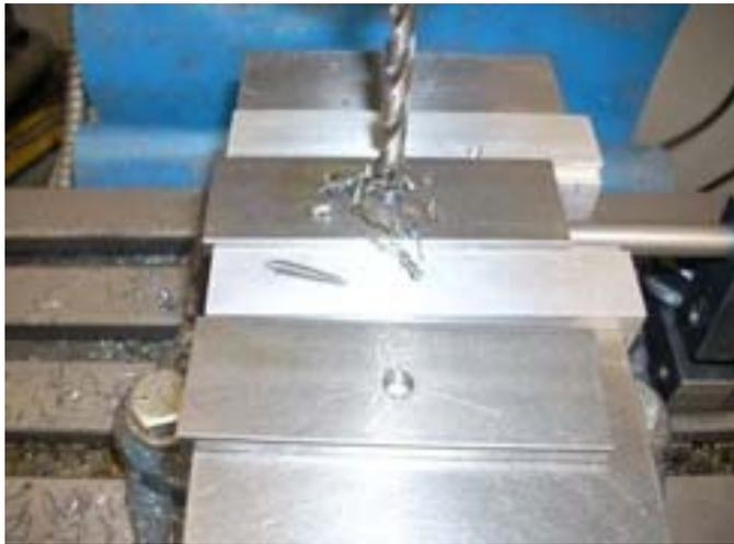
**Drilling Alignment Hole** Photo by R. G. Sparber
