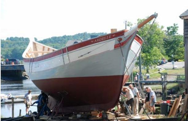
The ship is built on a framework that extends into the water at high tide. The keel is laid on a series of blocks called dry blocks, that are arraigned securely on the framework and construction commences. The ship is built up to and including the deck. The various final fitting out and stepping of the masts are finished after the ship is in the water.
