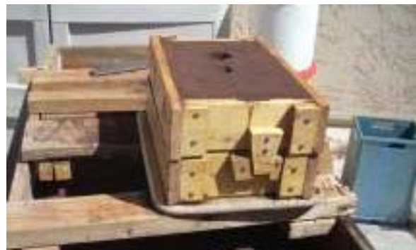
Ramming up Next Flask Photo by R. G. Sparber
