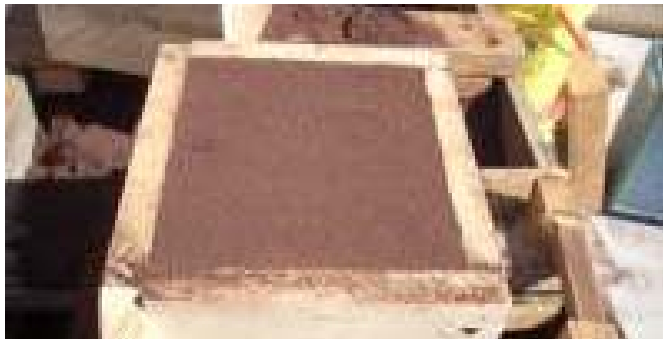
Bottom Struck Off Photo by R. G. Sparber
