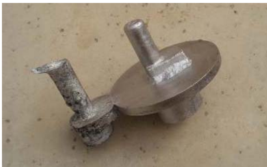
Sprue and Riser Photo by R. G. Sparber
