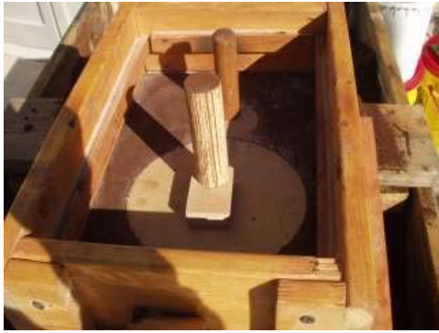
Sprue Fitted to Gate Photo by R. G. Sparber
