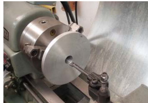
Boring for Bushings Photo by R. G. Sparber
