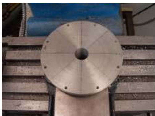
Bolt Holes Drilled Photo by R. G. Sparber
