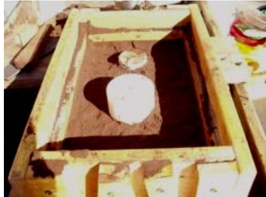
Casting in Petrobond
