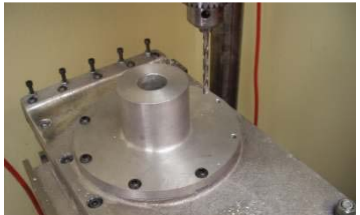
Mounting Bearing Support Photo by R. G. Sparber
