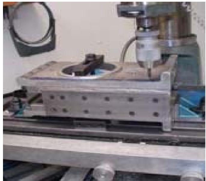
**Center Drilling Casting Photo by R. G. Sparber**
