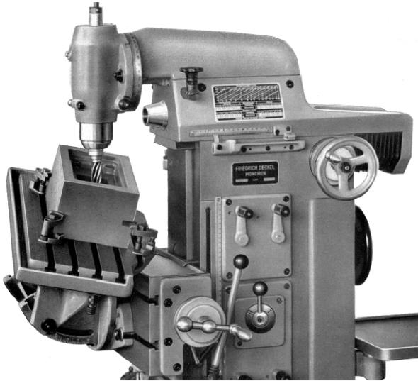
Catalog photo of a Deckel FP-1 in use, showing the unique capabilities of a universal mill
