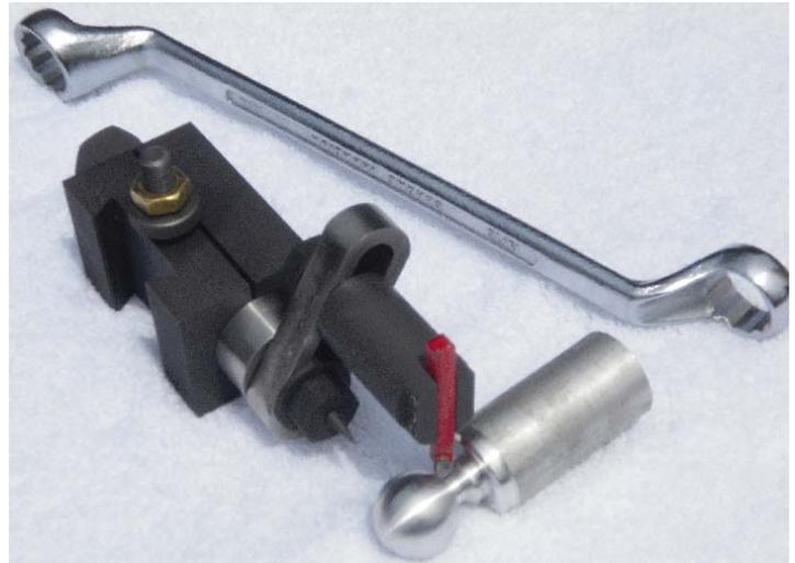
bolts, washers, threaded rod, setscrews, an E-clip, and an O-ring. If you already have a 1" Aloris style boring bar holder, you need only make 4 parts: Shaft, Spacer, Swing Arm, and Tool Bit Holder. Details for machining those parts are shown in the drawings below.
