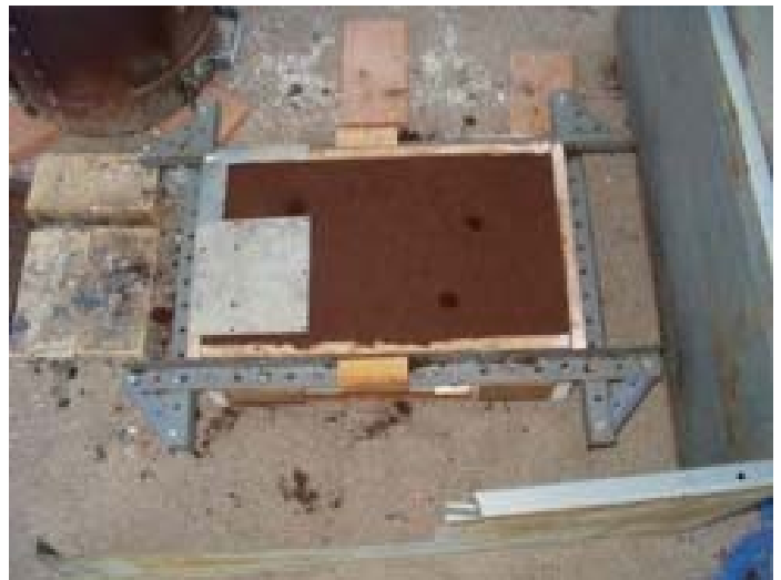
Steel Frame on Cope Photo by R. G. Sparber
