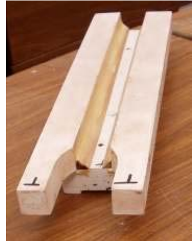
Front Column Pattern Photo by R. G. Sparber
