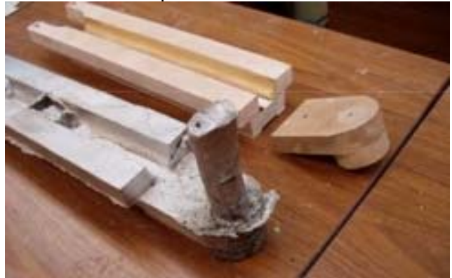
Sprue Gate & Pattern Photo by R. G. Sparber
