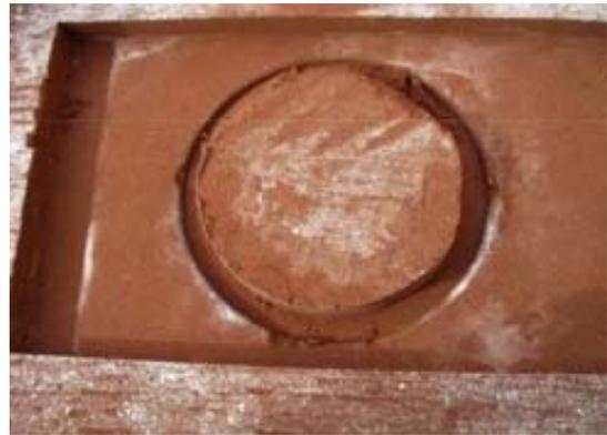
With the pattern drawn, you can see some damage to the edge around the hole. I did not ram hard enough. On my second casting with this pattern, I rammed much harder. I used my narrowest tool and worked the sand into the pattern at a 45-degree angle. It greatly reduced this problem.
