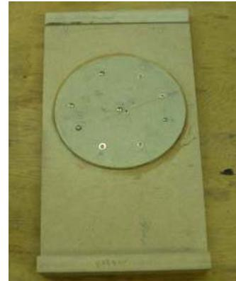
Above is the pattern before I cut the hole. One lesson learned is to write lots of instructions on the pieces to be glued together. The draft is only 1 to 5 degrees and it is easy to stick a piece of wood on upside down. It also prevents me from using a finished strip of wood as a glue spreader.
