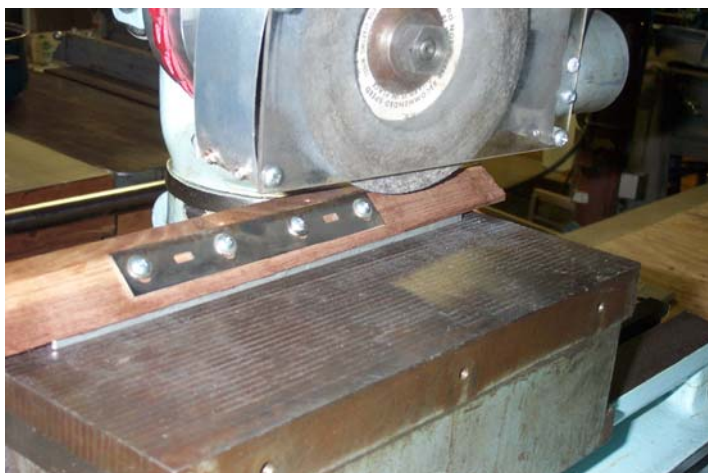
Jointer knife held in a wooden fixture on a LeBlond No. 1 Universal Grinder
