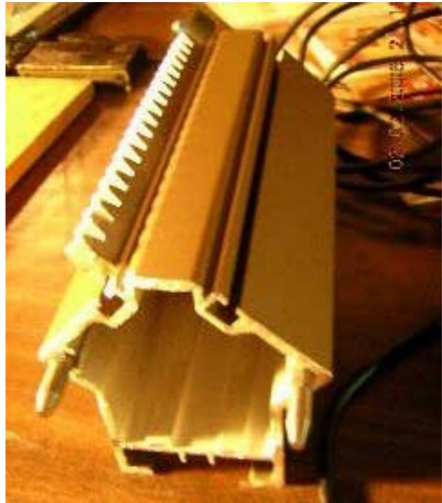
The straight stairlifts are based on an aluminum extrusion with a rack (see picture), mounted to the steps. The arms of the chair and the footrests are linked. Raising the arms folds up the footrest.
