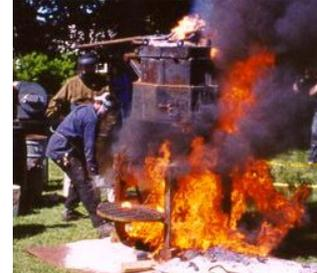
necessary to cast the molds that are prepared and are on the foundry floor. After the firing was completed and the slag cleaned out of the copula, the bottom was dropped and the remaining coke was
