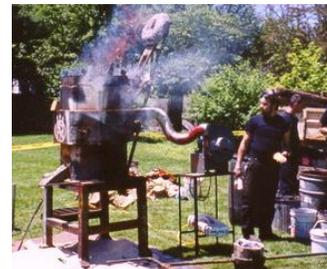
material has been applied to the inside as a lining with a band of holes leading from a plenum chamber into the furnace proper. These holes are called tuyeres (pronounced
