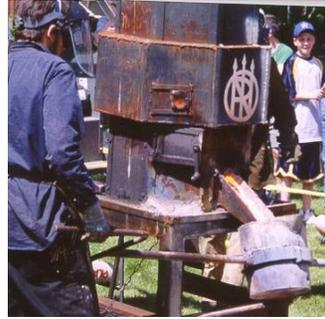
enough molten iron, a second bot was placed in the tap hole. The slag was scooped from the iron, the ladle was carried over to the molds and the pour into the mold commenced.
