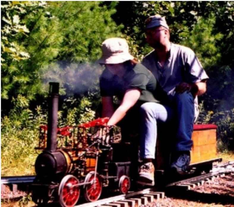
← Here we see another distinctive locomotive, a model of a very early “Grasshopper” engine. The cylinders are mounted vertically at the rear of the engine, and operate the red levers visible on the top of the engine. The lever is pivoted at the front of the engine. The connecting rods to the wheels are in between. This means that the stroke of the cylinder is larger than the throw of the crankpin on the wheels.
