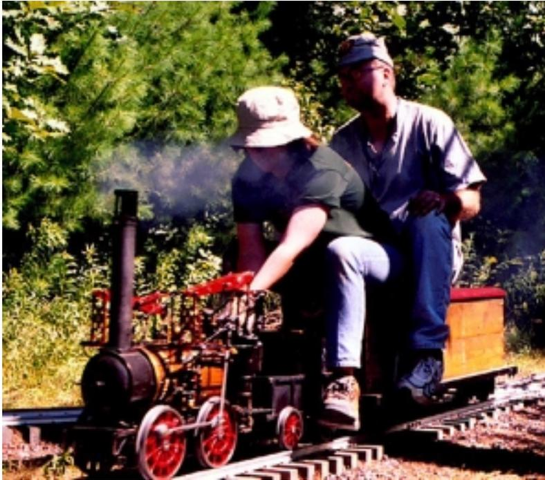
← Here we see another distinctive locomotive, a model of a very early “Grasshopper” engine. The cylinders are mounted vertically at the rear of the engine, and operate the red levers visible on the top of the engine. The lever is pivoted at the front of the engine. The connecting rods to the wheels are in between. This means that the stroke of the cylinder is larger than the throw of the crankpin on the wheels.
