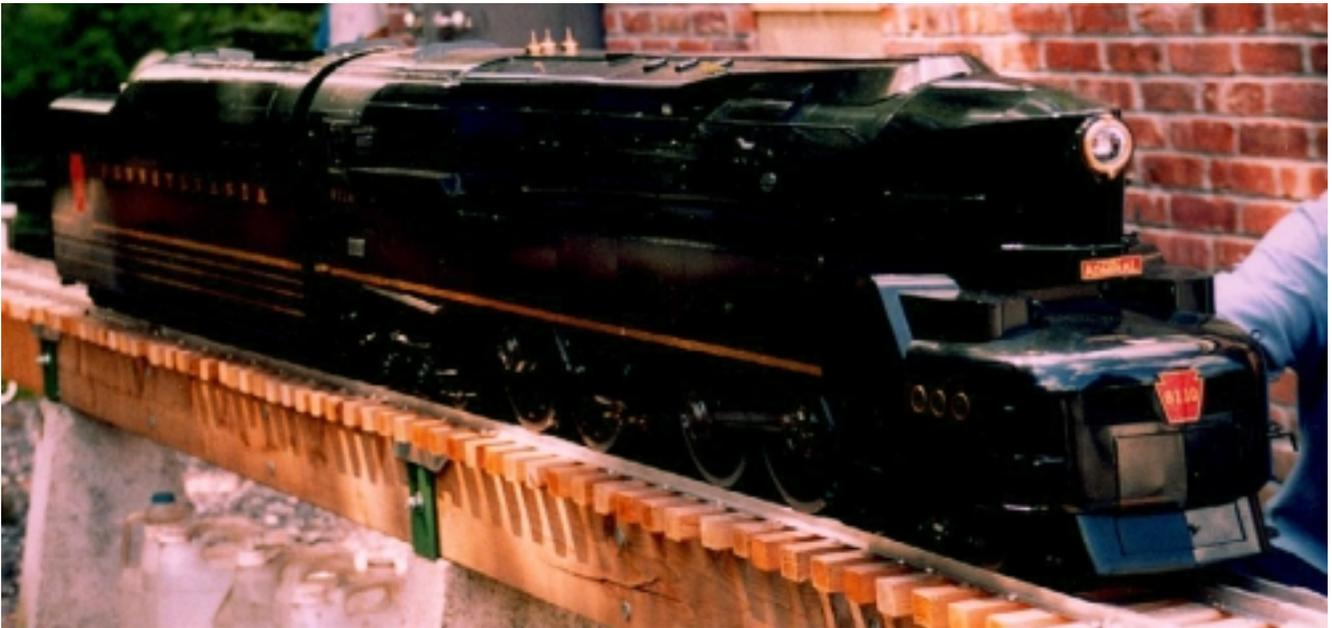
↑ For me, one of the highlights of the meet was seeing Ed Wooding's 1" model of a Pennsylvania Railroad T-1 class 4-4-4. The Pennsy experimented with a variety of wheel arrangements towards the end of steam. One of the more successful was the T-1. They built 2 for testing, and liked it enough to build 48 more, with minor modifications. This engine is unique in that while it has four cylinders, each pair powering two drive axles, it was a rigid frame. This was known as a "Duplex" arrangement.
