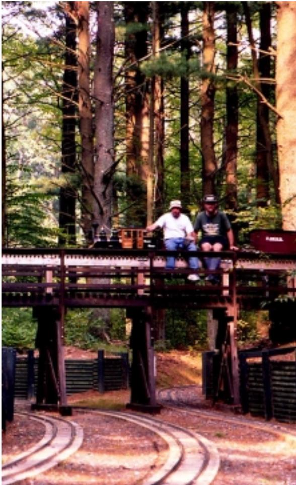
↑ Here we see Pat Fahey crossing “Dimond Trestle” over the ground-line tracks. The engine is a 4 ¾” gauge model of one of the “Maine Two Footers”, 2 foot gauge prototypes which ran in rural Maine. Several of these engines survived to run at Edaville, in Carver, MA
