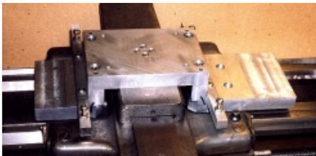
Mery Engine fixture on lathe carriage Norm Jones photo
