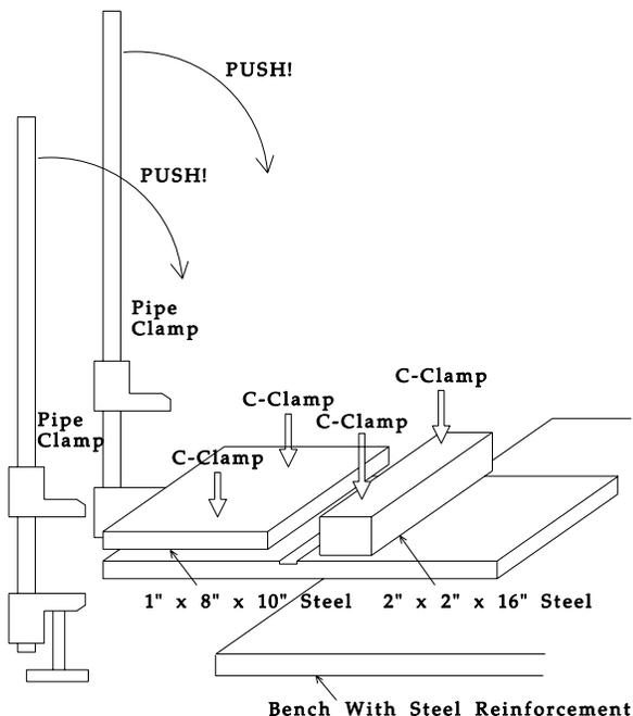
I clamped two pipe clamps onto the edge of the work, and pushed pretty hard. AMAZING! It started to bend! Push some more, and it bent some more. After a while, it wouldn't go any more, because I was pushing at a funny angle and clamps were hitting other clamps, so I flipped the pipe clamps over. Now, instead of pushing forward and down, I was pulling back and pushing up. That gave me the extra swing space to complete the bend.
