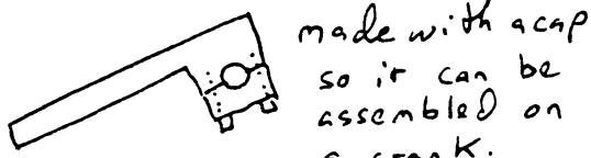
When the fit on the shaft gets loose and needs to be tightened, take the cap off and rub it on 320 paper, then put it back together. The removable cap lets you lap the crank journal where you couldn't get to it with a lap with only one split.
