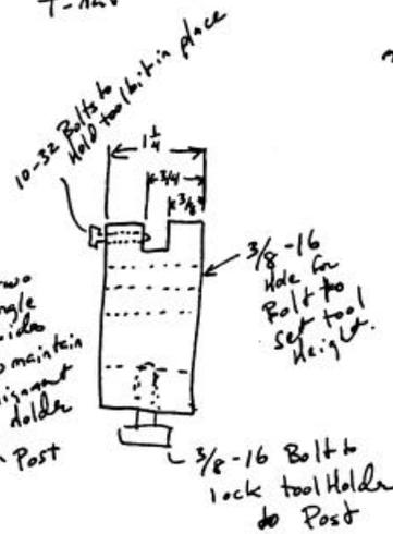
To make Angle guides: mount stock coupling nut.
