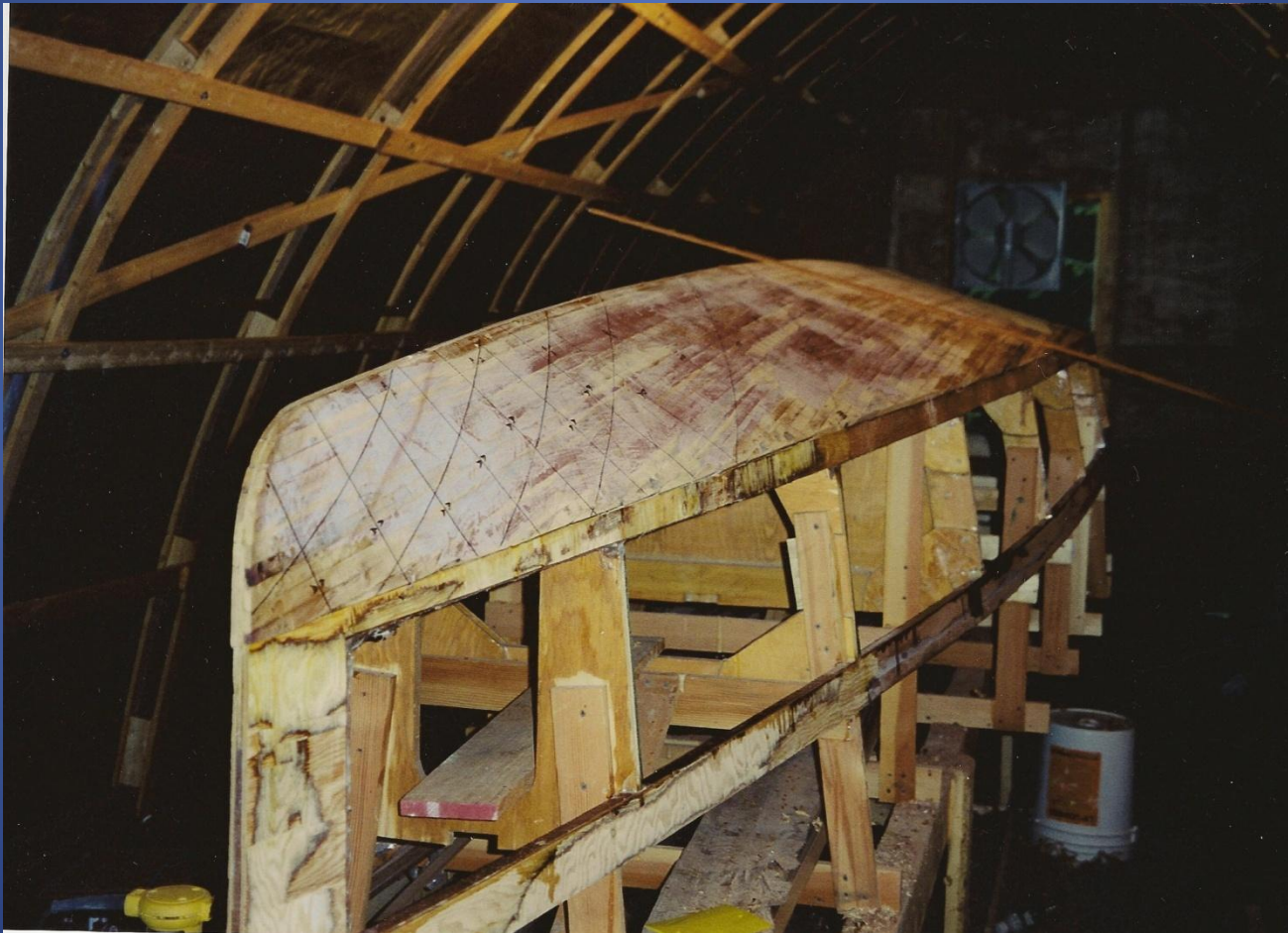
Lining out for the cold molded layers and checking fairness
