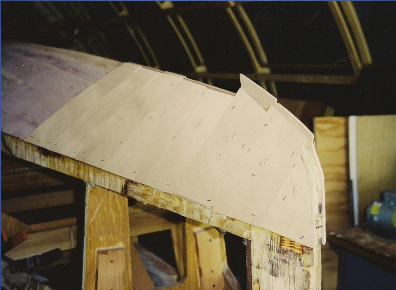
Dry fitting plywood strips prior to numbering and gluing
