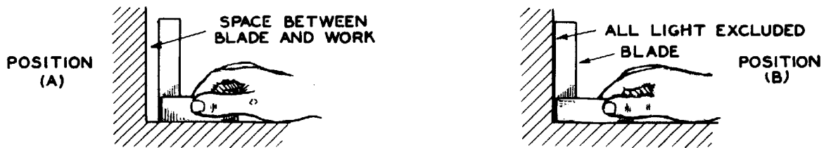
FIG. 19 TESTING AN INSIDE RIGHT ANGLE FOR SQUARENESS
