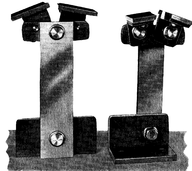
Fig. 5A Showing the construction of the Rest
