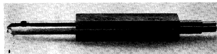
Fig. 7 Holder for keyway cutting tool
