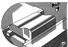
Often the form of the contour is laid out on the end of the piece, and, when this is the case, it is the duty of the operator to manipulate the work and the tool so that the finished surface conforms to the contour line. The contour may be produced in one of the following ways.
