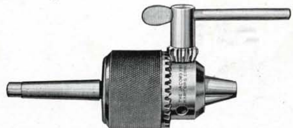
Fig. 20—Drill Chuck on Taper Shank
