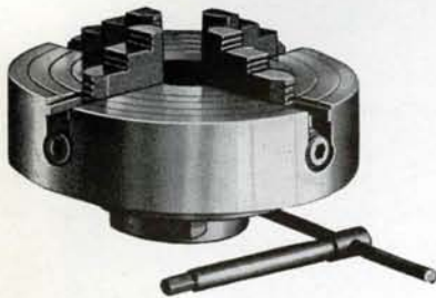
Fig. 16—Six-inch—Four-Jaw Independent Chuck
