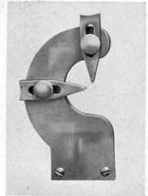
Fig. 22. Follower Rest. Attaches to base of slide rest. Used when threading or turning slender work on centers. Brass jaws, 3" dia. capacity
