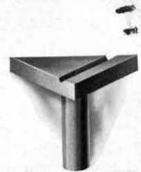
Fig. 22. Follower Rest. Attaches to base of slide rest. Used when threading or turning slender work on centers. Brass jaws, 3" dia. capacity
