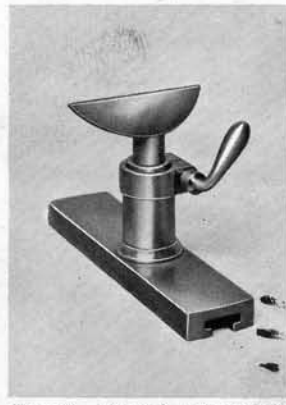
Fig. 24. T Rest. Mounts on lathe carriage in place of compound slide rest. Convenient for hand-tooling and wood-turning
