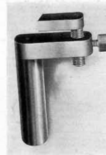
Fig. 25. L Rest. Mounts in T rest base in place of T. Valuable for hand-tooling in narrow grooves and corners and truing work held in jaw chuck
