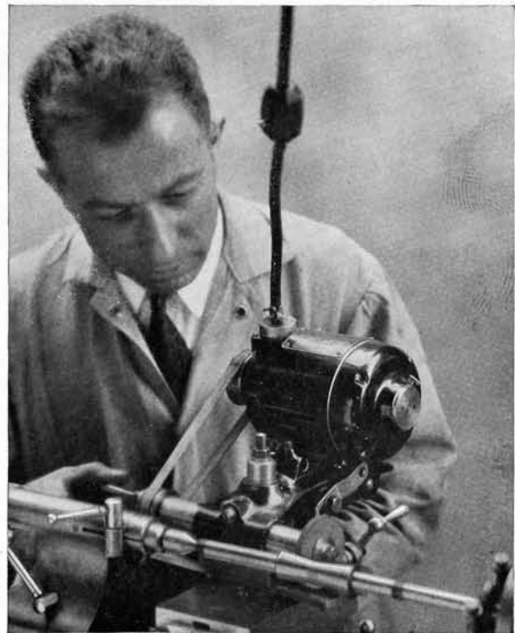
Fig. 9. Unit Motor Drive Slide Rest Grinding Attachment mounted on top slide of rocker tool post slide rest with external quill (rear view), grinding taper on shaft
