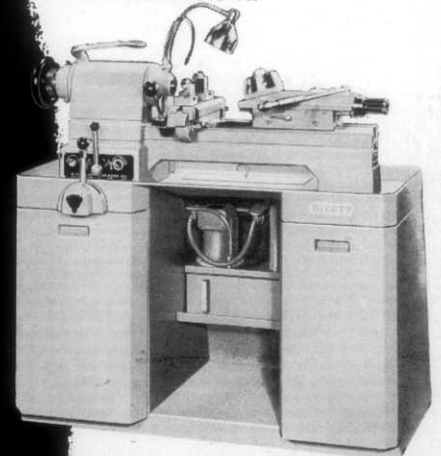
Rivett Model 918 "Steelway" Turret Lathe. 9" swing, 20" between collet and turret face, 1⅛" draw-in, or 1⅝" stationary collet capacity. Write for Bulletin 918-ST.
