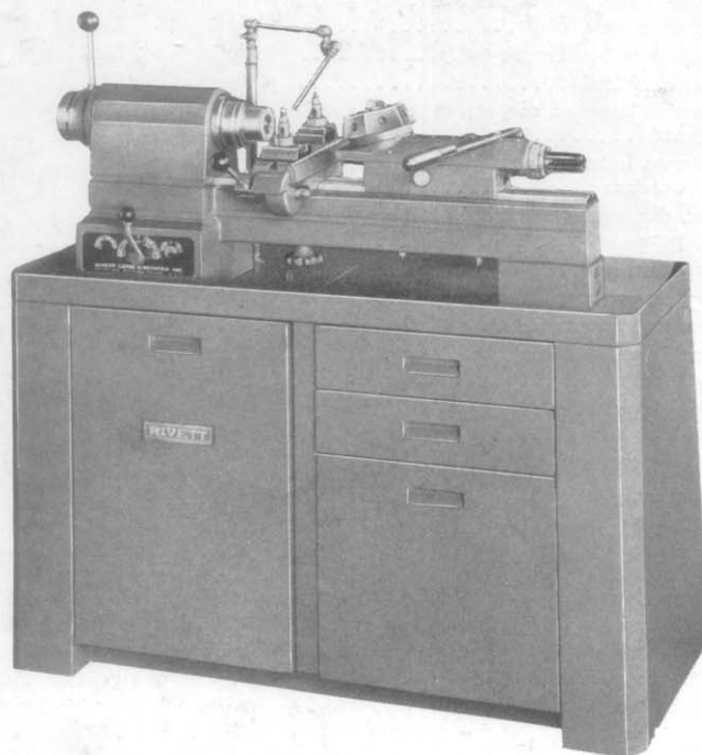
Rivett Series 918 Ball Bearing Hand Screw Machine on Metal Cabinet with Motor Jackshaft Drive. Collet Capacity 1"', Swing 9"', Bed 39 \frac{1}{2} ". Also furnished as plain Lathe.
