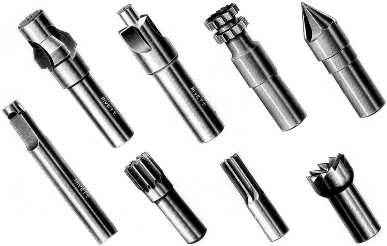
SAMPLES OF MILLS AND COUNTERBORES MADE ON THE RIVETT LATHE.
