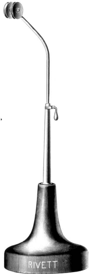
LEADER FOR OVERHEAD BELTING, for use with Grinding Attachment.
