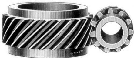
SAMPLES OF SPIRAL GEARS CUT ON THE RIVETT PRECISION LATHE.
