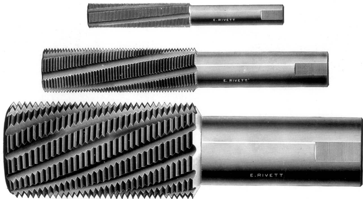
SAMPLES OF SPIRAL MILLING, HOBS, TAPS, Etc.
