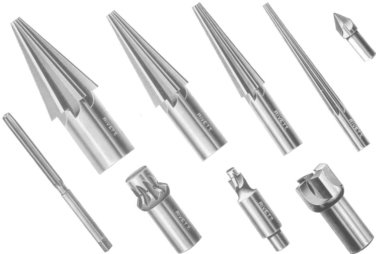
SAMPLES OF TAPER MILLS AND REAMERS MADE ON THE RIVETT LATHE.
