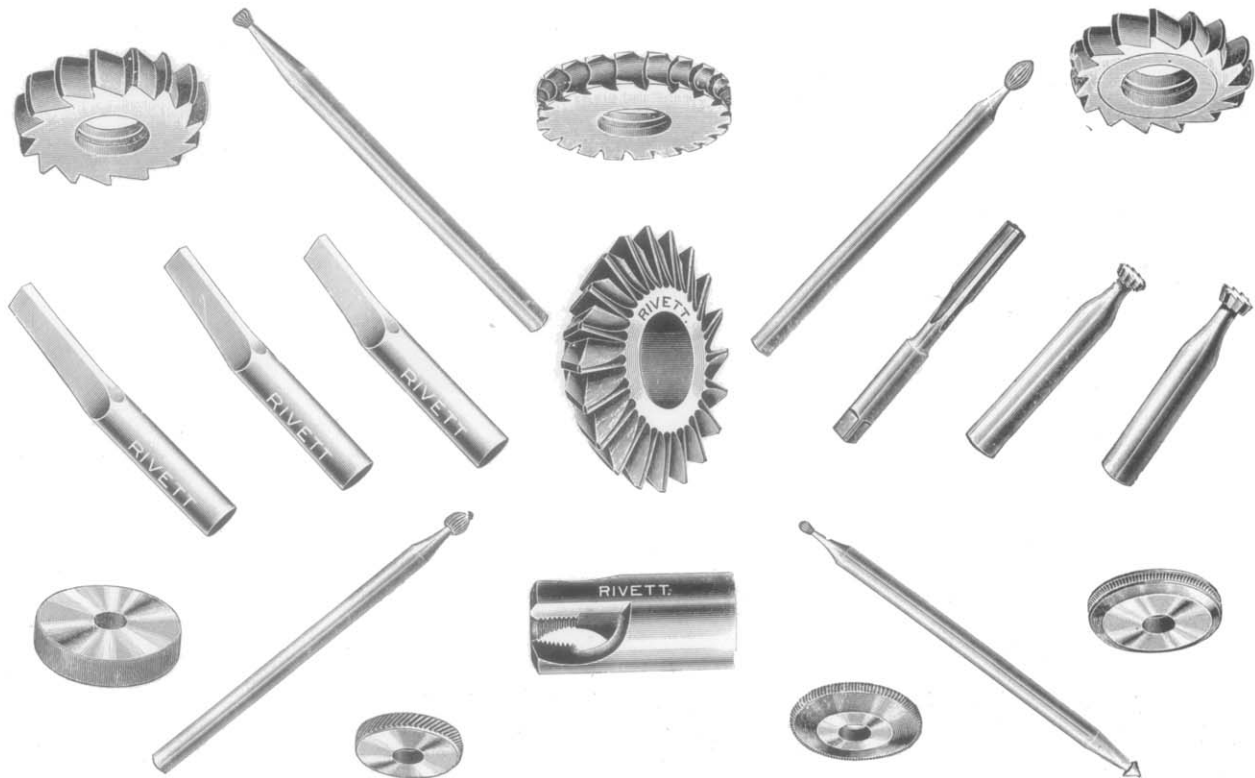
Some of the finest Knurls ever made for watch case work, etc., are made on the Rivett Lathe.
