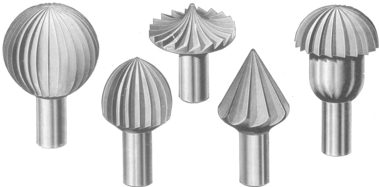
Samples of IRREGULAR MILLING CUTTERS made on the Rivett Lathe, using only the Attachment as shown on page 26.
