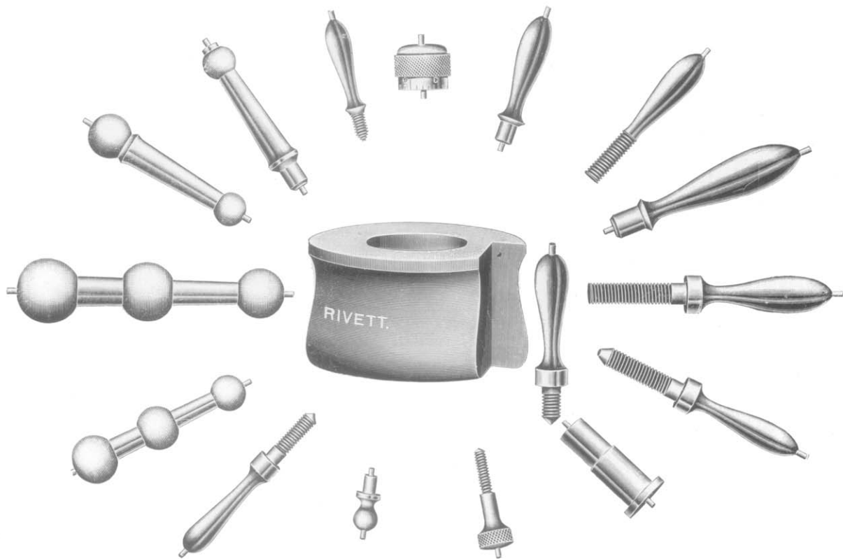
SAMPLES OF FORMING SLIDE WORK.
