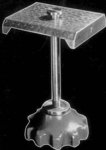
Fig. 6 - Shoe with Clamping Bolt and Knob
