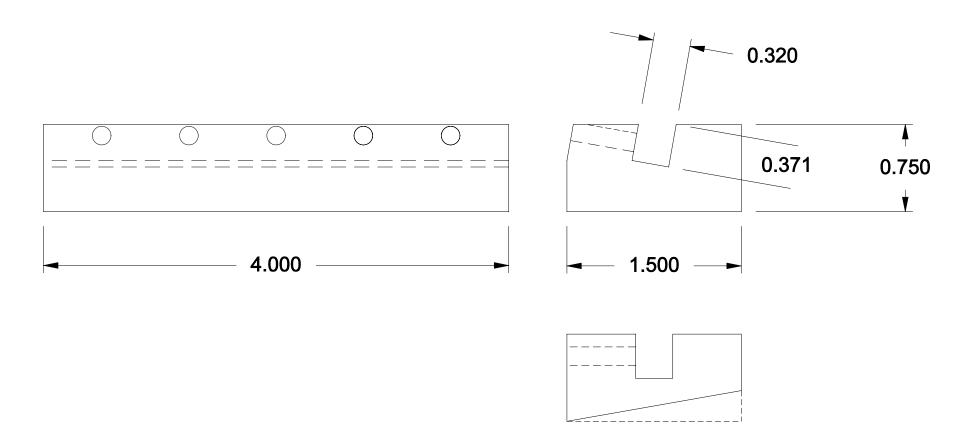
Alternate construction. Mill slot and drill and tap holes, then mill bottom to desired angle
