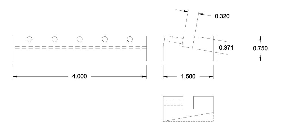
Alternate construction. Mill slot and drill and tap holes
