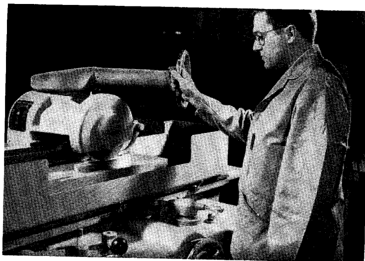
Norton 6" Surface Grinder, using 8 x 1/2 x 1 1/4" wheel
