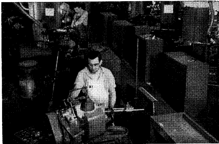
A well laid-out tool grinding department. Note large drill grinder in foreground
