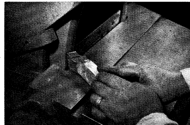
Hold the tool lightly against the Crystolon wheel and keep moving the tool constantly to avoid overheating it
