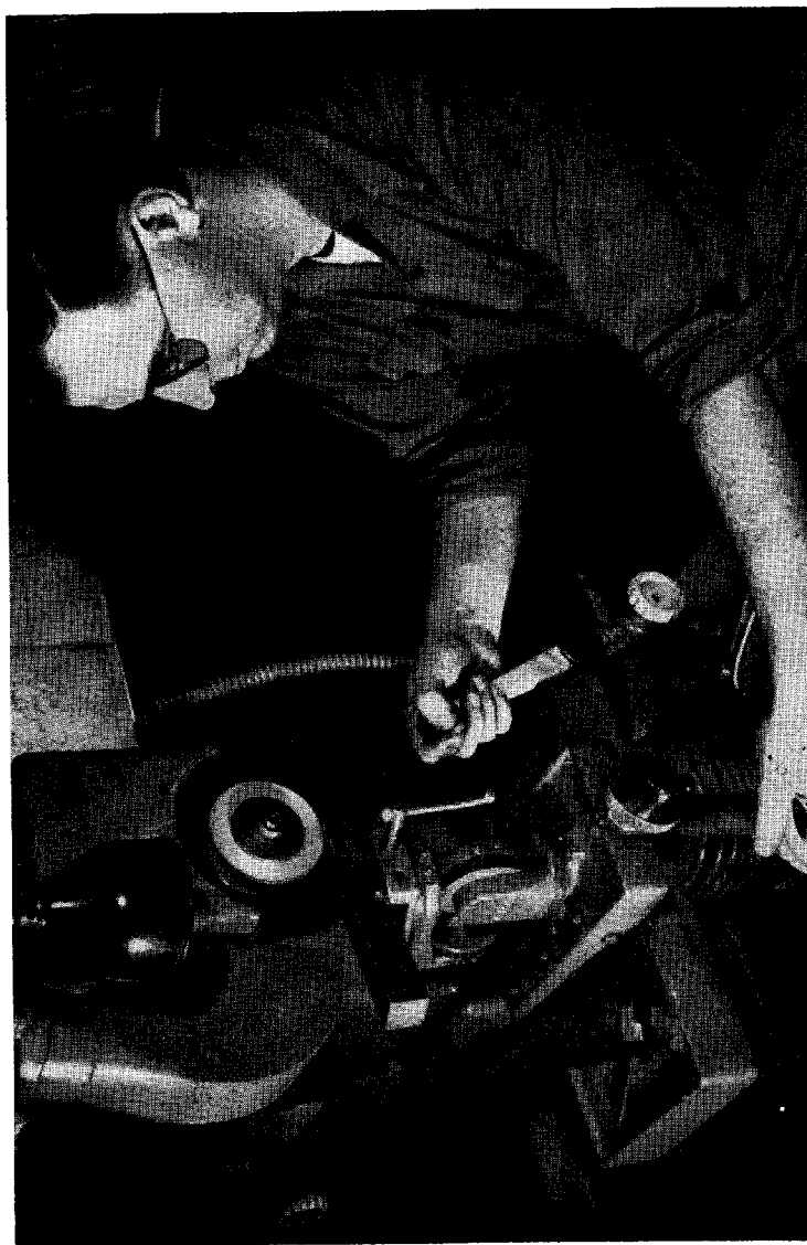
Grinding a chip breaker with a durable SD150-R100B1 1/8 resinoid bonded diamond wheel
