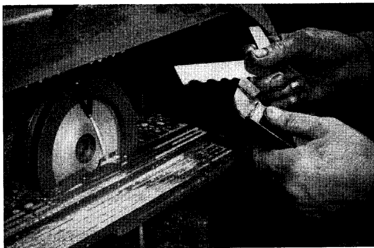
The nose radius should be accurately ground and blended into the side and front cutting edges
