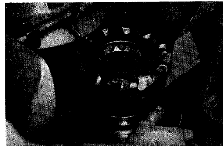
Sharpening a carbide inserted blade face mill on a special cutter grinder equipped with a type DIA1 (DIT), 150 grit diamond wheel
