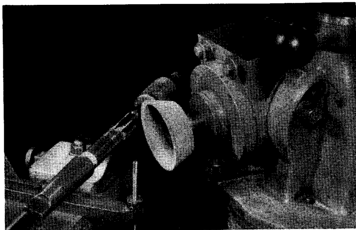
Sharpening a machine reamer by backing off the front cutting edges (wheel guard removed to show set-up details)
