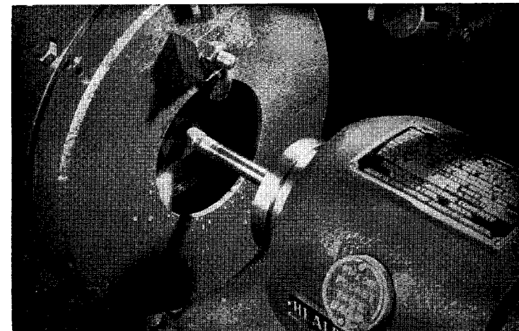
Bore grinding a carbide die with a vitrified bonded diamond wheel
