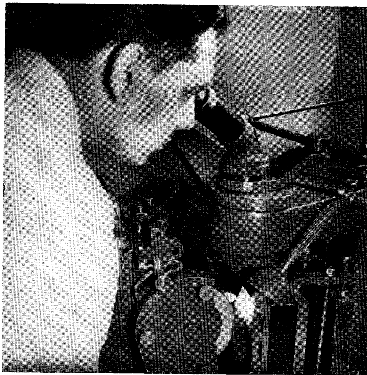
Grinding the contour of a flat form tool on an optical type precision form tool grinder equipped with a 220 grit diamond wheel
