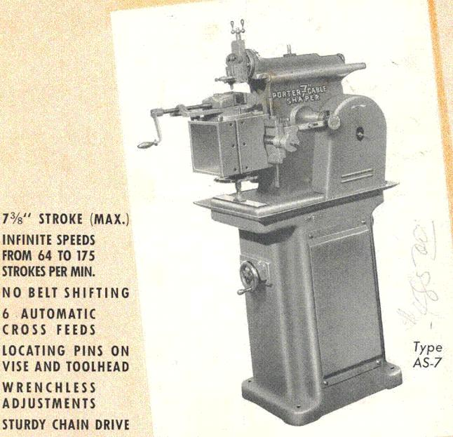
INFINITE SPEEDS FROM 64 TO 175 STROKES PER MIN. NO BELT SHIFTING 6 AUTOMATIC CROSS FEEDS LOCATING PINS ON VISE AND TOOLHEAD WRENCHLESS ADJUSTMENTS STURDY CHAIN DRIVE OPERATES FROM 1/2-H. P. 1725 R.P.M. MOTOR IN BASE
